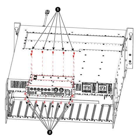
Image 14-74 E2 Gen 2 - Genlock assembly removal
