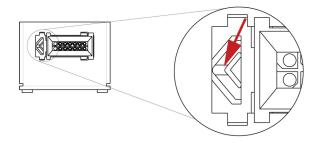
4. Push the connector to the left until the slots in the metal bracket align with the flanges on the connectors.
