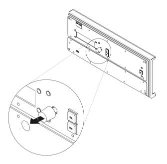
2. Use the knob removal tool provided by Barco to take out the knob. Align the notches on the tool with the grooves in the knob as indicated below.
