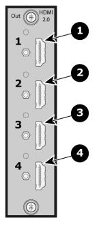
Image 4–16 Quad HDMI 2.0 Output Card Rear Panel
