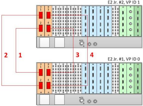
Image 6-60 Cabling between two E2 Jr. units
