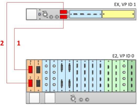
Image 6–49 Cabling between an E2 unit and an EX unit with a VPU card
