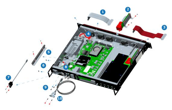
Image 16-19 Motherboard removal - chassis elements removed
