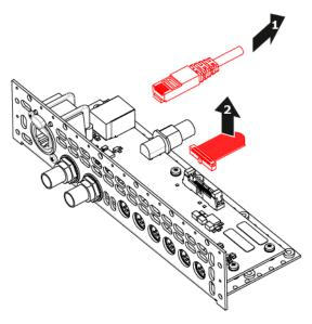
Image 14-75 E2 Gen 1 - Genlock assembly cables
