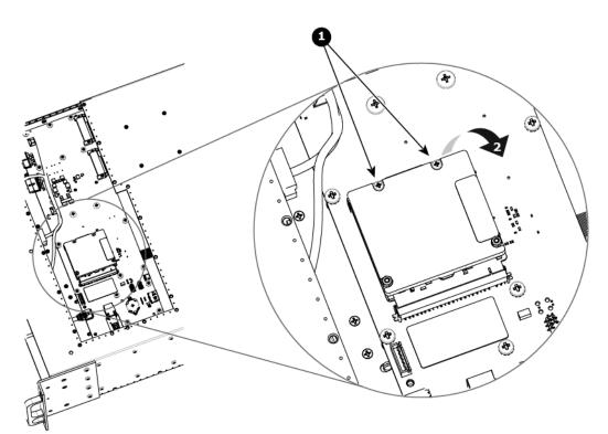
Image 14-58 CPU module removal - E2 Gen 2
