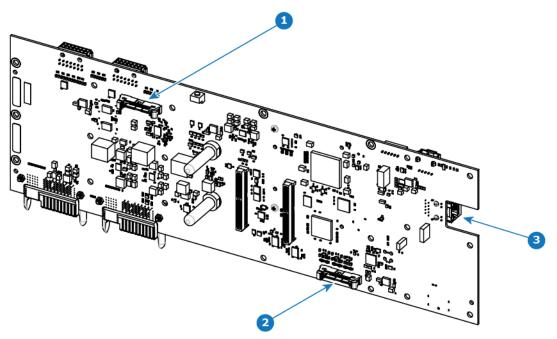
Image 14-69 E2 Gen 2 system power board - bottom side
