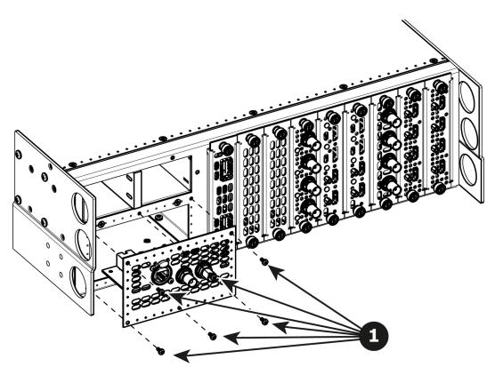
2. Gently pull the Genlock assembly away from the unit . Don't pull the assembly too far back because there are still 2 cables attached.
