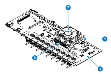
Image 15-53 S3 Q7 CPU motherboard with fan
