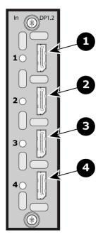
Image 4–11 Quad Channel DisplayPort 1.2 Input Card Rear Panel
