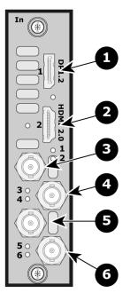
Image 4–13 Tri-Combo Input Card Rear Panel
