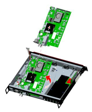
Image 16-21 Motherboard removal - removing the motherboard
