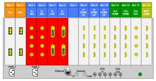
Image 6-15 E.g. E2 with an empty input-card slot
