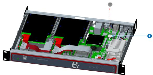
Image 16-15 System battery removal
