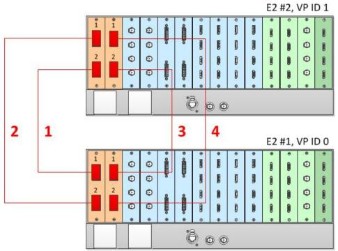
Image 6-45 Cabling between two E2 units
