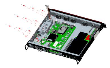
Image 16-20 Motherboard removal -motherboard screws
