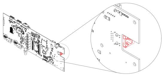
Image 14-92 Ethernet-cable connector
