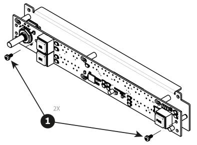
2. Move the PCB to the right and then out to release it from the mount.
