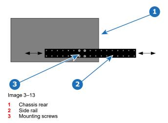
3. Re-install the mounting screws. When properly adjusted, the end of each side rail will protrude through the slot in the rear mounting bracket, once the chassis is rack mounted.
