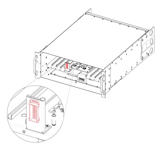
3. Locate the snap lock on the top of the connector and push it back to release the connector from the bracket.
