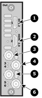
Image 4–18 Tri-Combo Output Card Rear Panel
