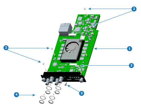
Image 14-16 Screws, standoff, washers, and nuts
