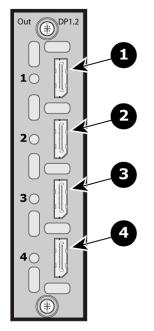
Image 4–14 Quad Channel DisplayPort 1.2 Output Card Rear Panel
