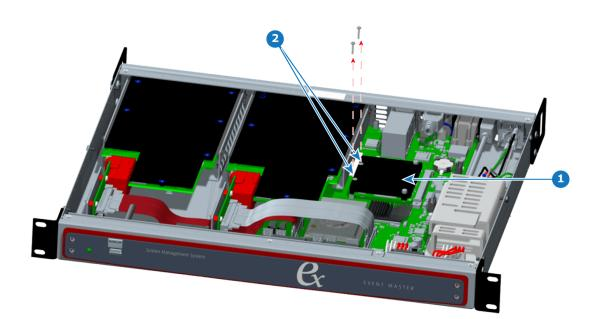
Image 16-12 CPU module components
