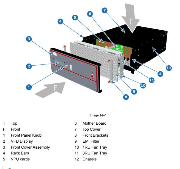
The EMI filter is no longer included or required. It should be removed.
