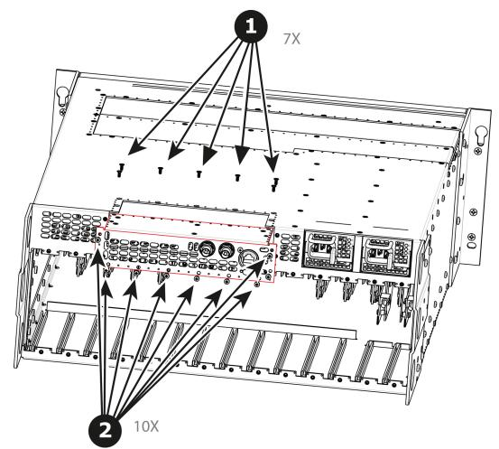
Image 14-73 E2 Gen 1 - Genlock assembly removal
