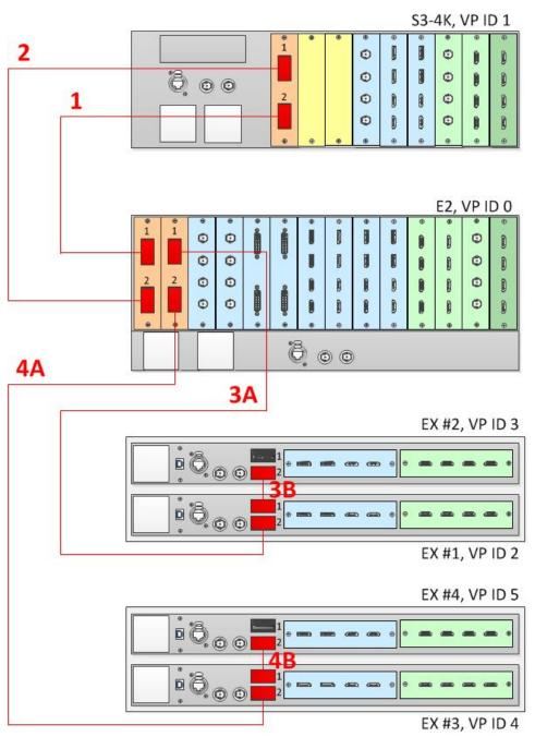
Image 6–54 Cabling between an E2 unit, an S3–4K unit, and four EX units
