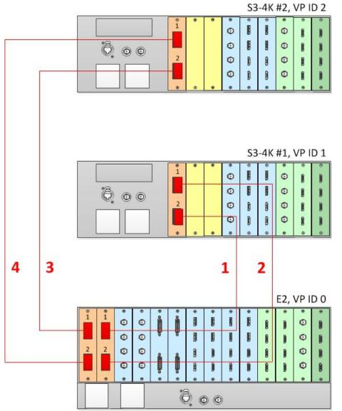
See Image 6–53 for an example of the cabling between an E2 unit and two S3-4K units.
