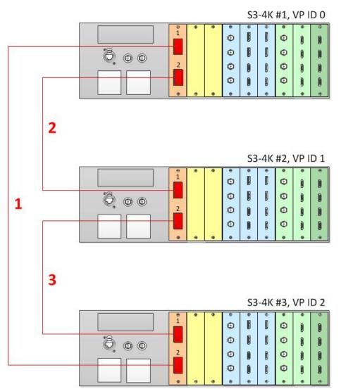
Image 6-55 Cabling between three S3-4K units
