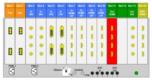
Image 6–19 E.g. E2 with an empty output-card slot
