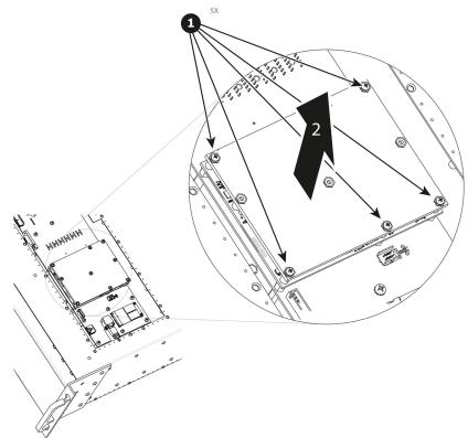
Image 14-57 CPU module removal - E2 Gen 1
