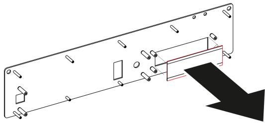
2. Use alcohol to clean the adhesive residue that held the filter to the metal plate.
