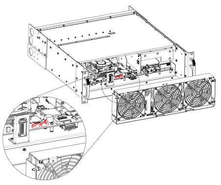
3. Pull the cable out of the unit .
