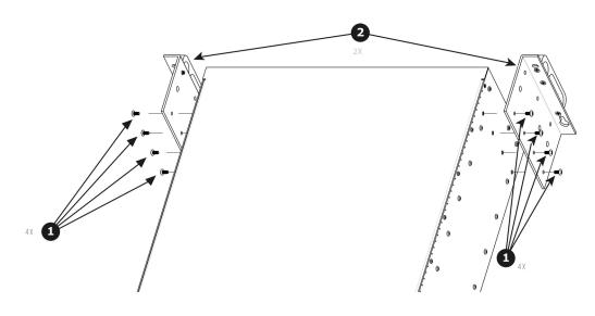
2. Remove the Rack-Mount Brackets from the Chassis.
