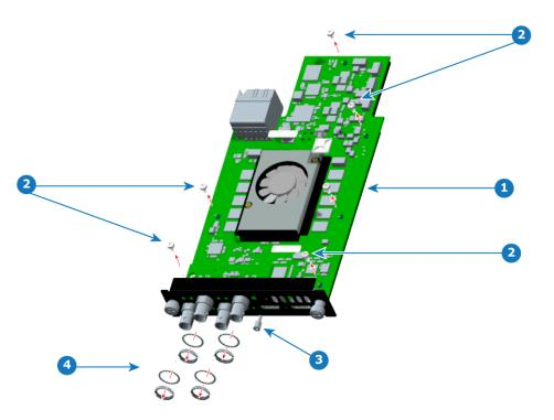
Image 14-9 Screws, standoff, washers, and nuts
