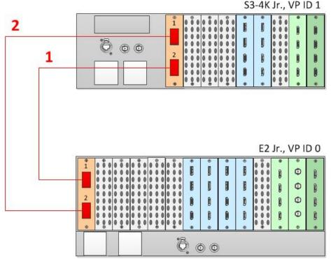
Image 6-62 Cabling between an E2 Jr. unit and an S3-4K Jr. unit
