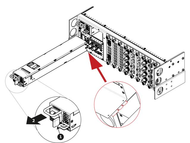
2. Pull the Power supply out of its slot by pulling on the handle.
