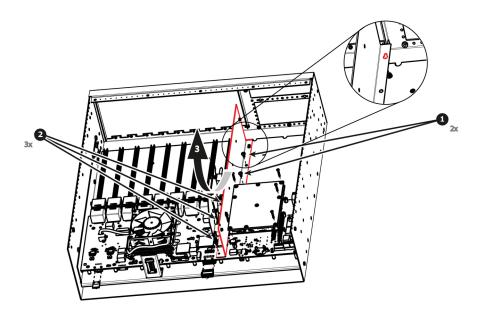
Note: It could be necessary to release the cable tie that maintain the fan power cable in place.
