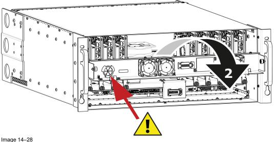
*Caution:* Before you completely remove it from the unit carefully push the USB and Front panel cables through the grommet located on the left hand side.
