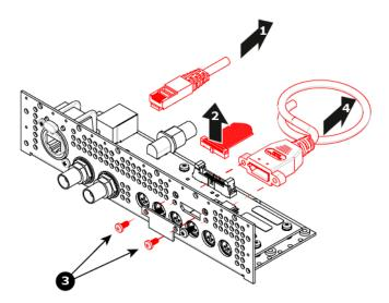
Image 14-76 E2 Gen 2 - Genlock assembly cables
