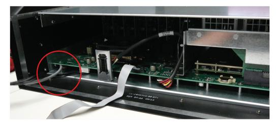
Image 15-35 USB Ext Cable connected to the Motherboard
