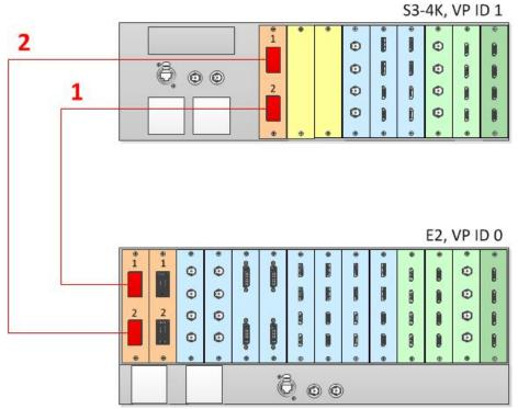
Image 6–52 Cabling between an E2 unit and an S3-4K unit
