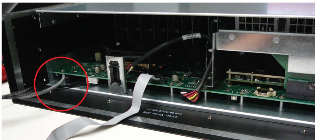
Image 14-34 USB Ext Cable connected to the Motherboard
