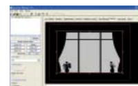
Bitmap masking: Detailed masking is also possible with an image of up to 1,920 by 1,200 pixels for the PT-DZ21K and 1,400 by 1,050 pixels for the PT-DS20K.
