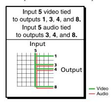
Figure 3-16 — Example 2, final configuration
