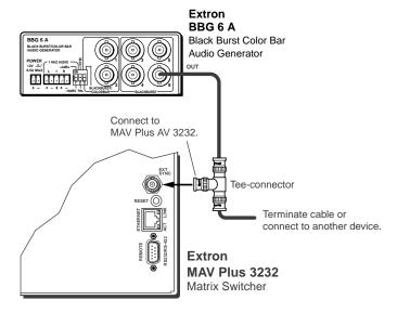
Figure 2-23 — Simple external sync connection example
