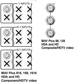
Figure 2-14 — MAV Plus component/HDTV video connections
