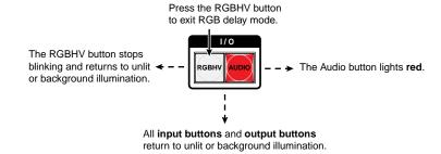
Figure 3-41 — Deselect RGB Delay mode
