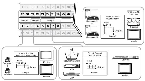
Figure 3-29 — I/O grouping of incompatible video formats
