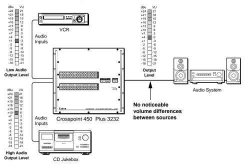
Figure 3-56 — Audio gain and attenuation
