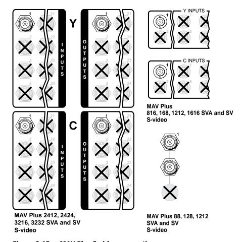
Figure 2-15 — MAV Plus S-video connections
