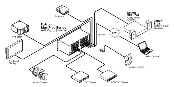
Figure 1-2 — Typical MAV Plus matrix switcher application
