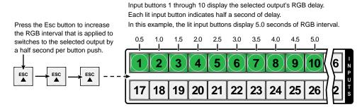
Figure 3-40 — Adjust the RGB delay interval
