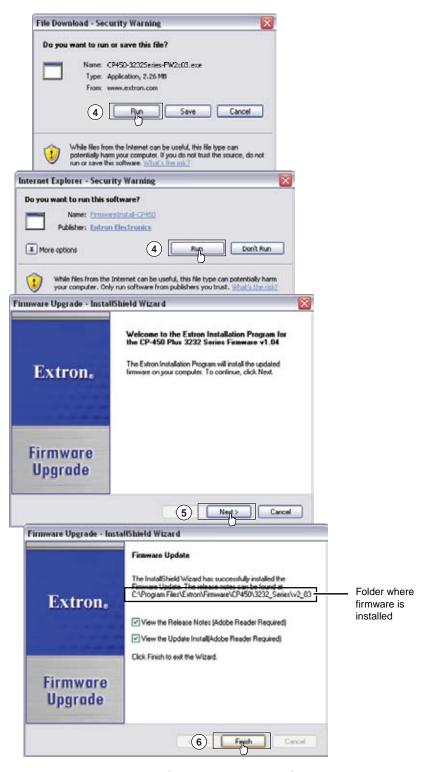
Figure 5-10 — Downloading firmware upgrade files
