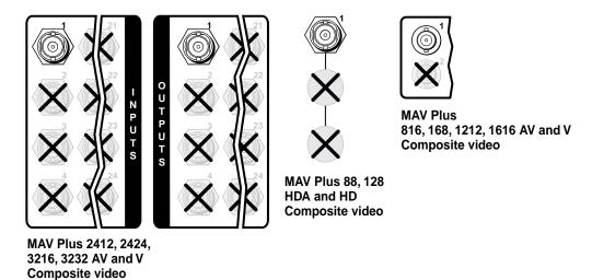
Figure 2-16 — MAV Plus composite video connections
