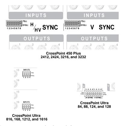
Figure 2-17 — Sync termination switches
