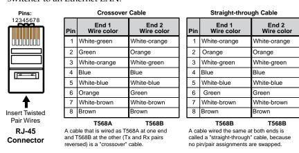
Figure A-1 — RJ-45 connector pinout tables
