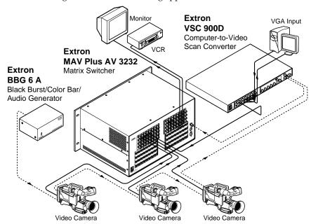
Figure 2-24 — Multiple device external sync connection example
