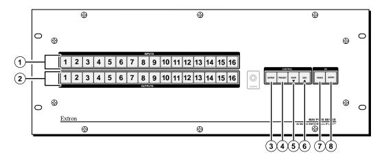
Figure 3-2 — Front Panel, MAV Plus 1616 HDA
