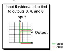
Figure 3-10 — Example 1, final configuration
