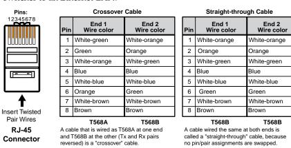
Figure 4-3 — RJ-45 Ethernet connector pin assignments
