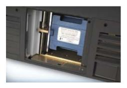
From 500W to 3.0W, the Christie Mirage Series features user-replaceable Xenon lamp modules with adjustable lamp power for lower brightness. The stable color temperature over the course of the lamp life and the power range provides the best lamp technology for color matching across multiple screens.
