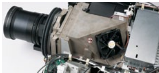
▲ Dust sealed engine
