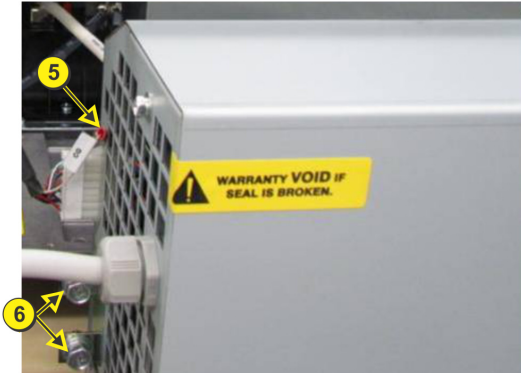
3.0kW and 2.4kW Ballast
