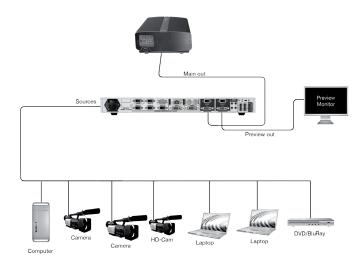
Connect all of your sources (PC, video camera, streaming server, DVD player...) to the appropriate input connectors at the rear of the unit (see "The **Pulse** rear panel" p.22 of the User Manual).
