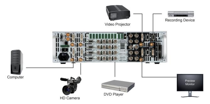
Connect all of your sources (PC, video camera, streaming server, DVD player...) to the appropriate input connectors at the rear of the unit (see "Input Specifications" p.14 of the User Manual).
