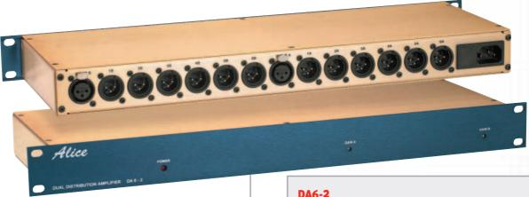
Stereo input to 6 stereo output distribution amplifier with input and outputs via XLR-type connectors. Suitable for stereo or dual mono distribution. May also be configured as 1-input, 12-output mono distribution amplifier by internal links.
