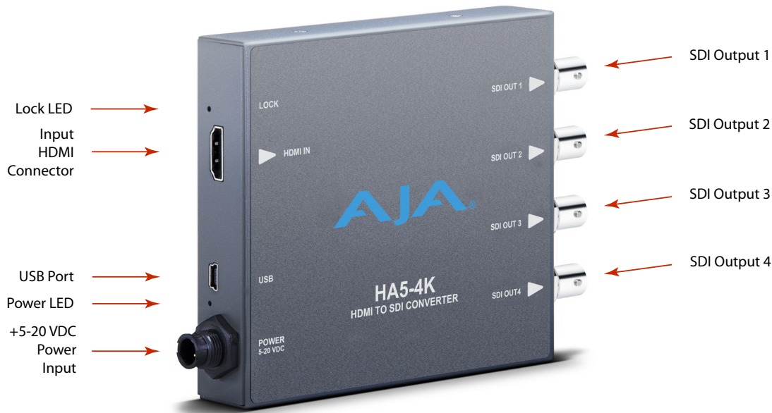
Figure 2. HA5-4K Converter Connections
